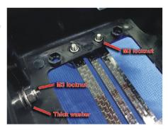
3) Use the M3x16mm screws to attach the links to the lower link mounts on your axles.
