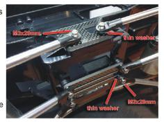
2) Make sure all screws are loosly in place before tightening down.
